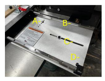
A- Miter slot Index pin for quick placement of tool and distance adjustment of slide table to cutter.
