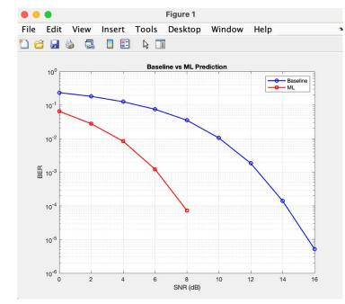
• ML out-performed traditional spatial channel estimation mapping one channel to another given two receivers in different locations.
