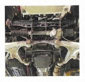
Call it an MGB reimagined. The Snake River Classics bodywork, including the optional fender flares, is subtle. Open the hood, though, for the big news: a modern, computer-controlled GM turbo-four. Modernization underneath includes an A-arm front suspension.
