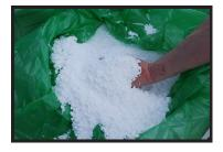
We also recycle EPS FORMPak back into packaging cubes (1/2" x 1/2" x 1") for use as a loose fill.
