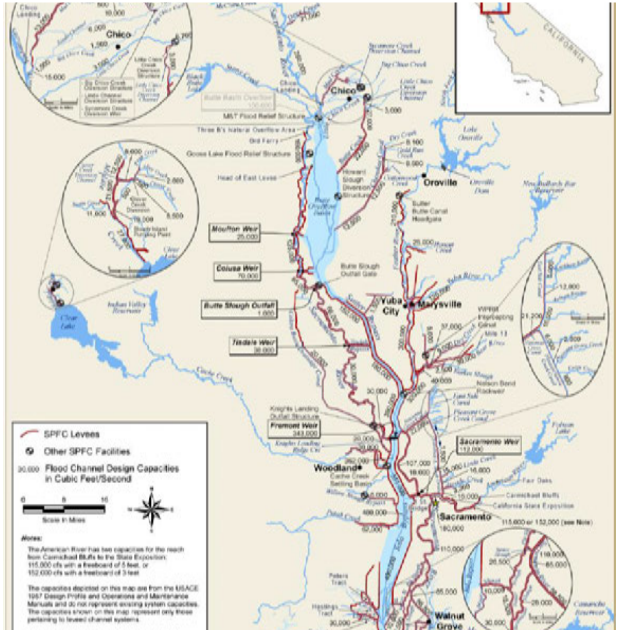
Figure 4. State Plan of Flood Control Facilities, Sacramento River Basin (DWR 2011)
