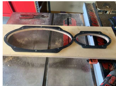
Opening trimmed to the template
