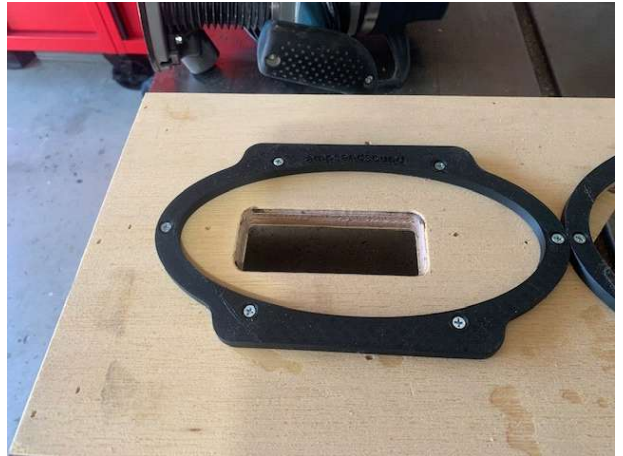
Template secured to the baffle
