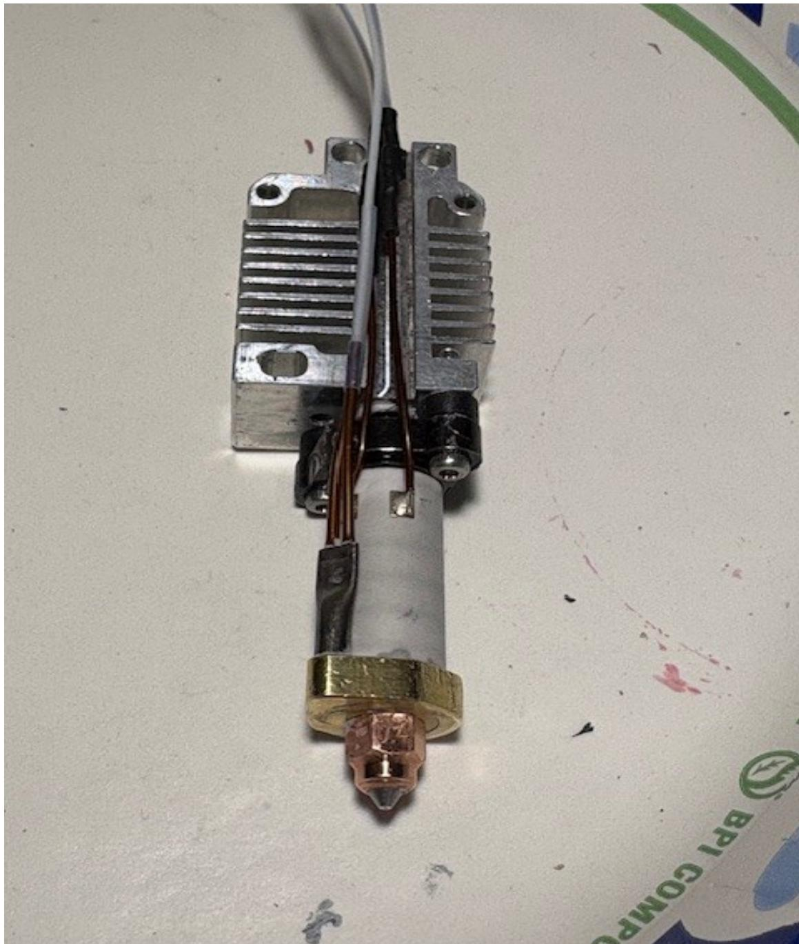
When assembly is complete it is a good idea to test the Thermistor should read approximately 1K ohms. It is also a good idea to check the installed height of the newly assembled hybrid Sovol Unicorn hot end. See photos below. The installed height is 75mm.
