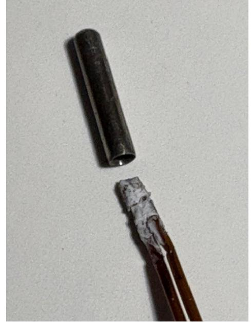
It is necessary to gut the Creality thermistor and save the sleeve to be re-used. I drilled the old thermistor out of the tip. Be cautious when drilling the thermistor sleeve. Sketchy
