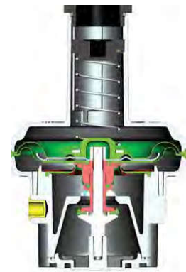
Standard Model Inlet Pressure Range: 3" W.C. to 2 PSIG
