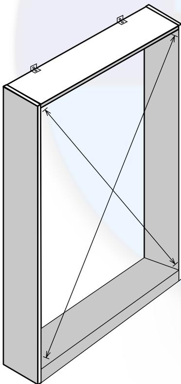
Before Installing the parts of the bed, make sure you have connected the cabinet to the wall, using the fixings provided. check diagonal across the cabinet to see if the cabinet is square.
