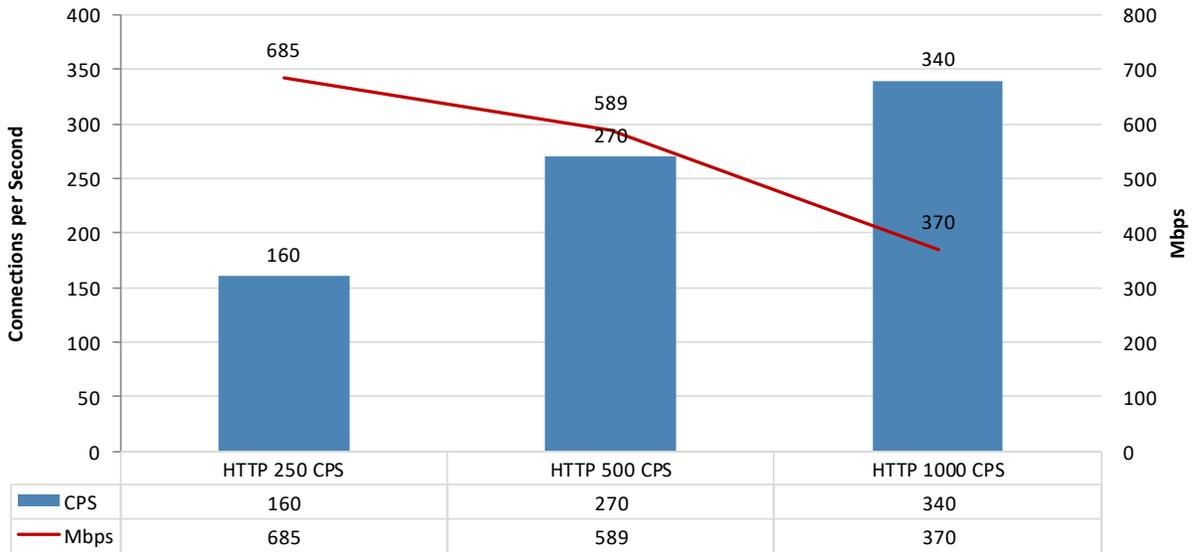
Figure 13 – HTTP Capacity with HTTP Persistent Connections
