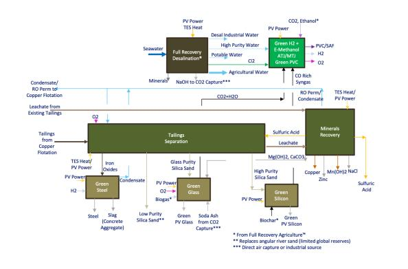
Figure 13 -- EWM Full Recovery Copper Tailings and Leachate Process<sup>™</sup> Block Flow Diagram
