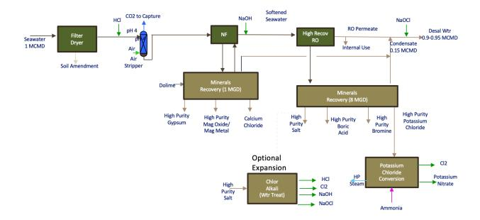
EWM Full Recovery Desalination<sup>®</sup> for Seawater. EWM integrates commercially proven technologies from multiple industries – no "unproven technologies" and no waste streams.
