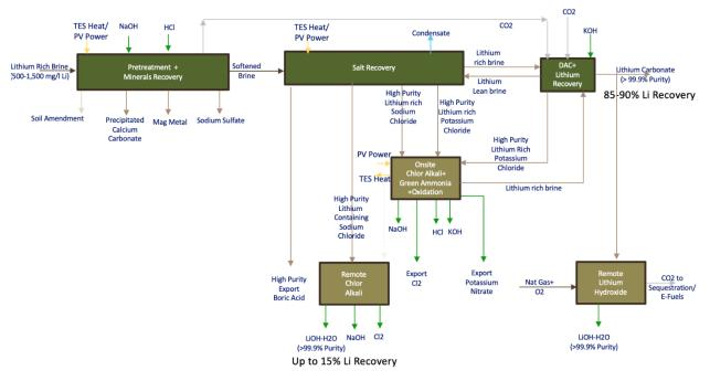
EWM Full Recovery Lithium Brine™ – 99% Lithium recovery with no "imported chemicals", no "waste tailings", and carbon capture from the atmosphere
