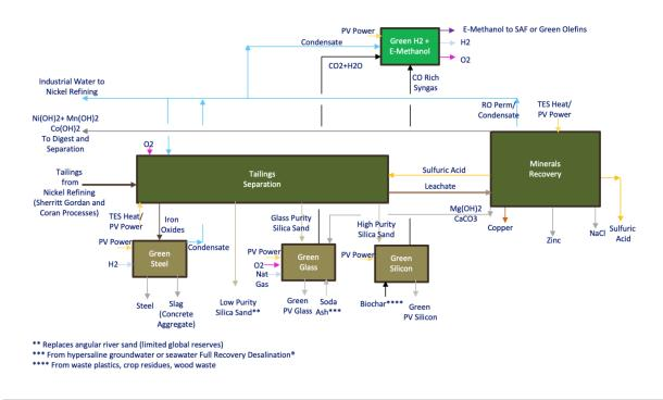
Figure 8 -- EWM Full Recovery Nickel Process<sup>™</sup> Block Flow Diagram for Tailings Minerals Recovery
