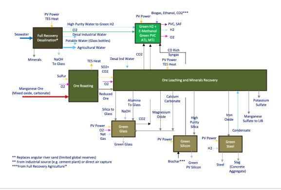
Figure 18 -- EWM Full Recovery Manganese Process<sup>™</sup> Block Flow Diagram
