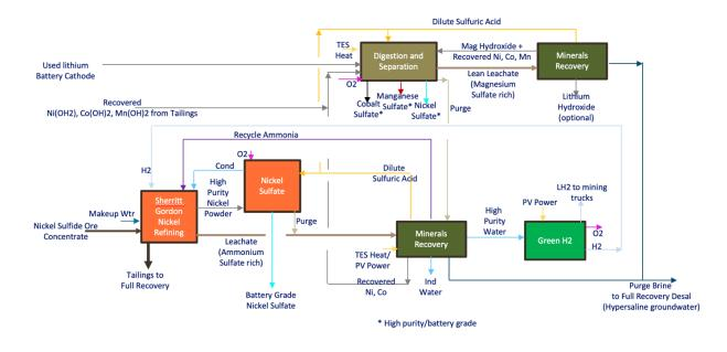
Figure 7 -- EWM Full Recovery Nickel Process<sup>™</sup> Block Flow Diagram for Primary Minerals Recovery – Nickel Sulfide Ore Concentrate
