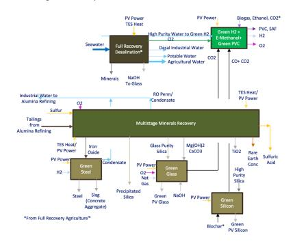
Figure 20 -- EWM Full Recovery Alumina Tailings Process<sup>™</sup> Block Flow Diagram
