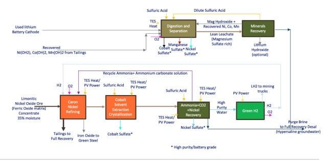
Figure 9 -- EWM Full Recovery Nickel Process<sup>™</sup> Block Flow Diagram for Primary Minerals Recovery – Limonitic Nickel Laterite Ore
