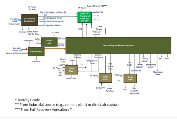
Figure 11 -- EWM Full Recovery Nickel Process<sup>™</sup> block flow diagram - Saprolitic Nickel Laterite Ore
