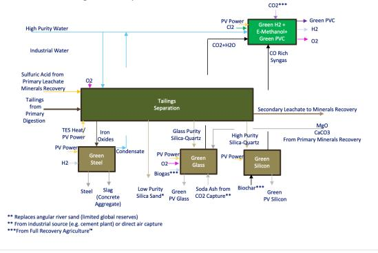
Figure 16 -- EWM Full Recovery Cobalt Process<sup>™</sup> Block Flow Diagram for Tailings Minerals Recovery
