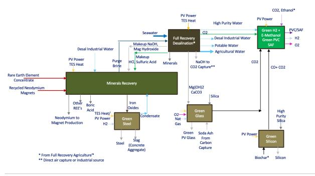
Figure 22 -- EWM Full Recovery Neodymium Process<sup>™</sup> Block Flow Diagram
