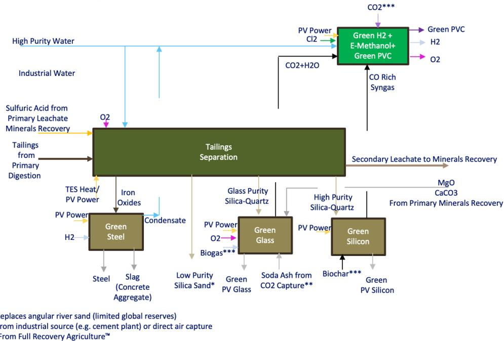
Figure 16 -- EWM Full Recovery Cobalt Process™ Block Flow Diagram for Tailings Minerals Recovery
