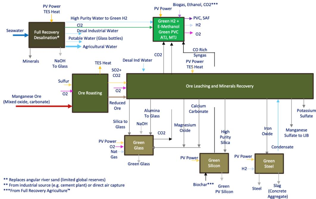
Figure 18 -- EWM Full Recovery Manganese Process™ Block Flow Diagram
