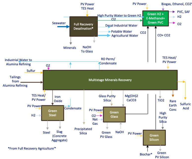
Figure 20 -- EWM Full Recovery Alumina Tailings Process™ Block Flow Diagram
