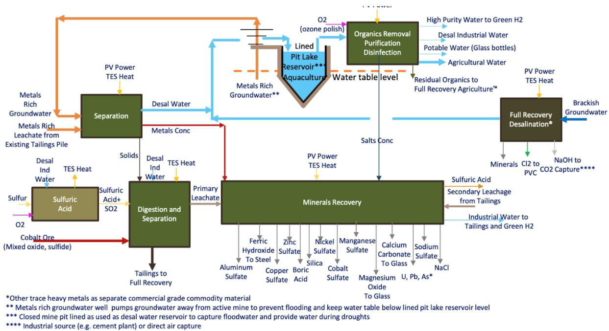
Figure 15 -- EWM Full Recovery Cobalt Process™ Block Flow Diagram for Primary Minerals Recovery
