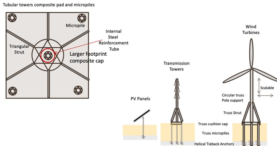
Figure 24 -- Conceptual Design of a PVC-glass Internal Steel Composite Based Micropile Foundation System is Shown for the Energy Transition Services (PV foundation, Transmission Line Foundation, and Wind Turbine Foundation)
