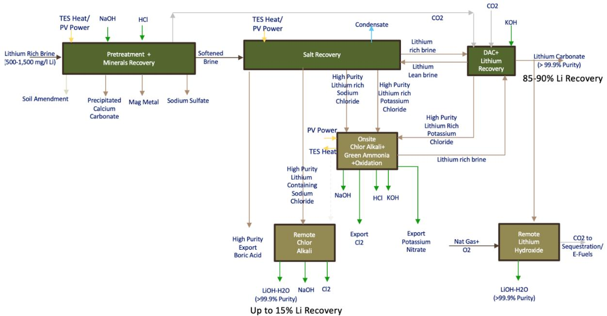
EWM Full Recovery Lithium Brine™ – 99% Lithium recovery with no “imported chemicals”, no “waste tailings”, and carbon capture from the atmosphere
