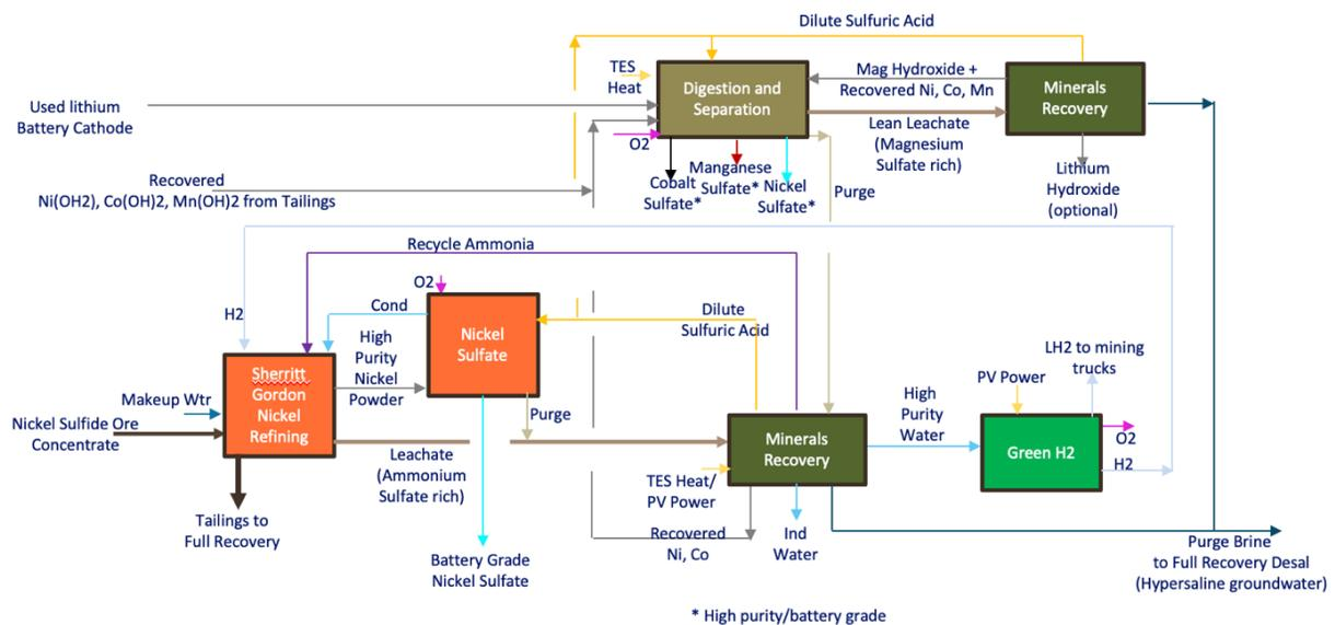
Figure 7 -- EWM Full Recovery Nickel Process™ Block Flow Diagram for Primary Minerals Recovery – Nickel Sulfide Ore Concentrate
