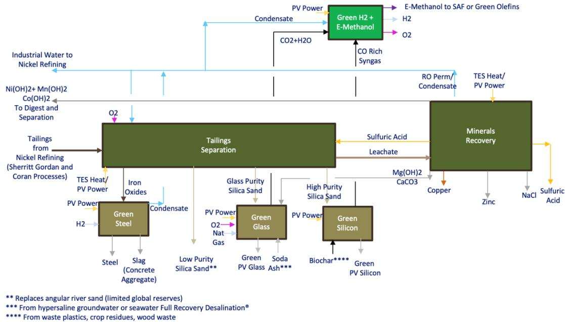
Figure 8 -- EWM Full Recovery Nickel Process™ Block Flow Diagram for Tailings Minerals Recovery
