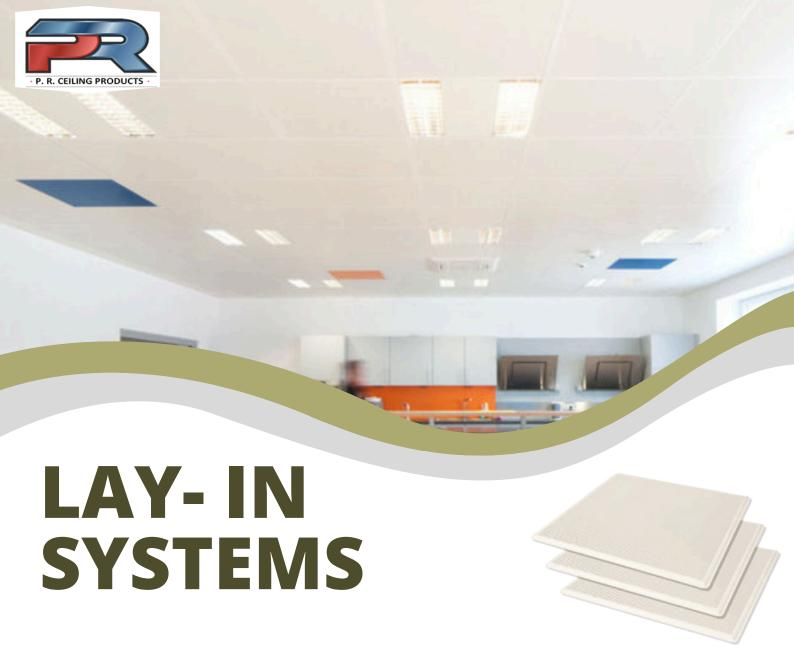
MCRA Lay-in false Ceiling System with steel/aluminum tile 595 mm X 595 mm is manufactured out of 0.50 mm thick polyester coil coated galvanized steel 120 gsm zinc coating or 0.7mm aluminum powder coated with 60 microns polyester paint in AA5050, AA3105 alum.
