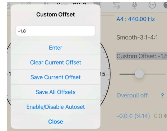
Tap on the offset text to manually enter a value, clear the offset or save the offset(s) as a custom offset in the tuning file and enable/disable auto set. In Auto set you might need to play the note a few times to settle the display to zero cents.
