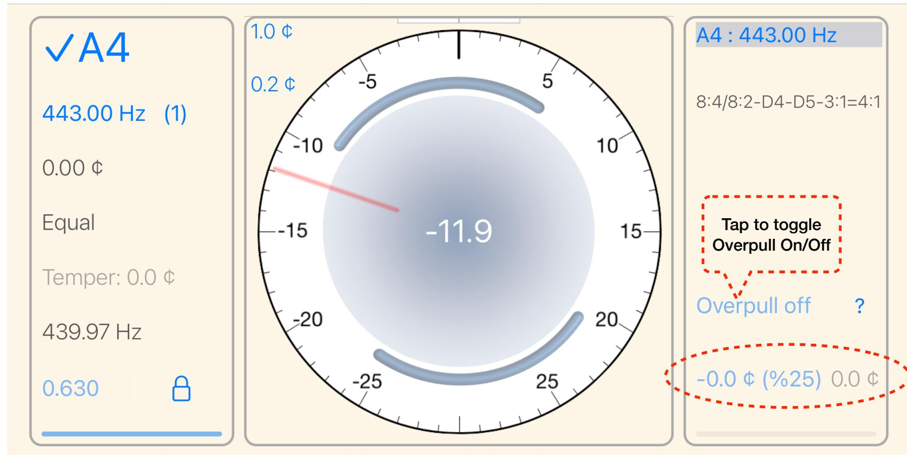
Observe the display when Over pull is ON, AND Over Pull Marker is set to OFF. Display shows that the note will be pulled by about 14.9 ¢ including the over pull amount.
