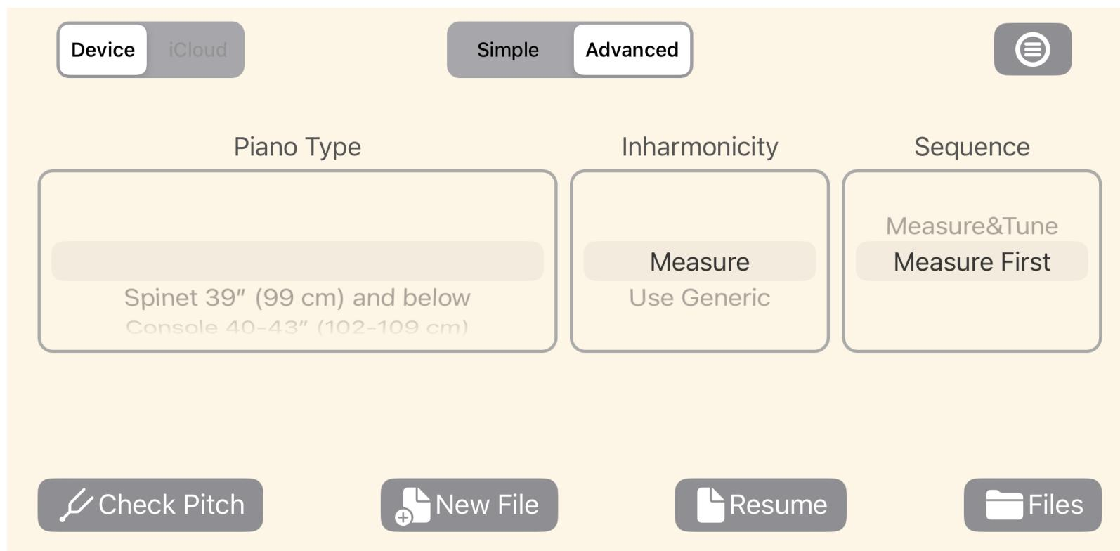
Check Pitch before tuning. You can add up to three markers on the check pitch scale which can be used for rough pitch raise. Select spectrum graph to rough tune open unisons.
