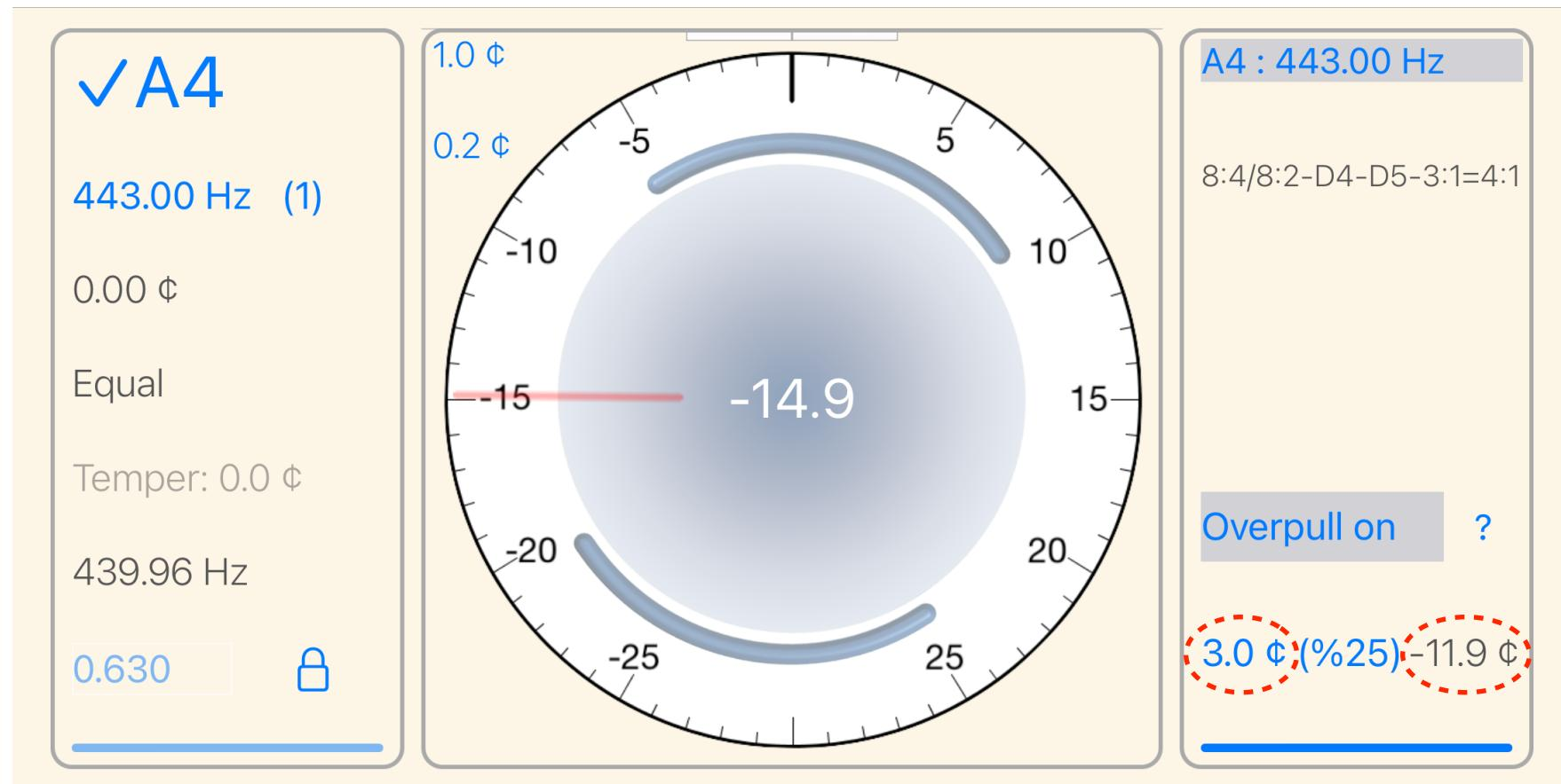
Tune as usual bringing the indicator close to zero. Note that measured frequency reflects the applied over pull amount.
