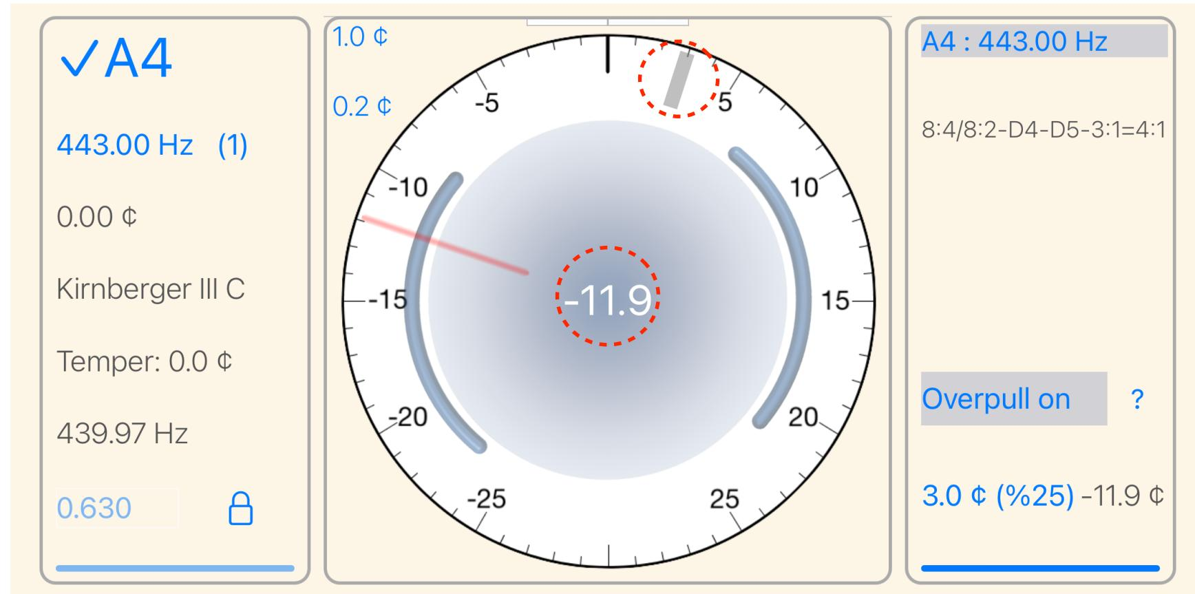
For over pull tuning tune the note to the marker. For normal tuning tune the note to zero.
