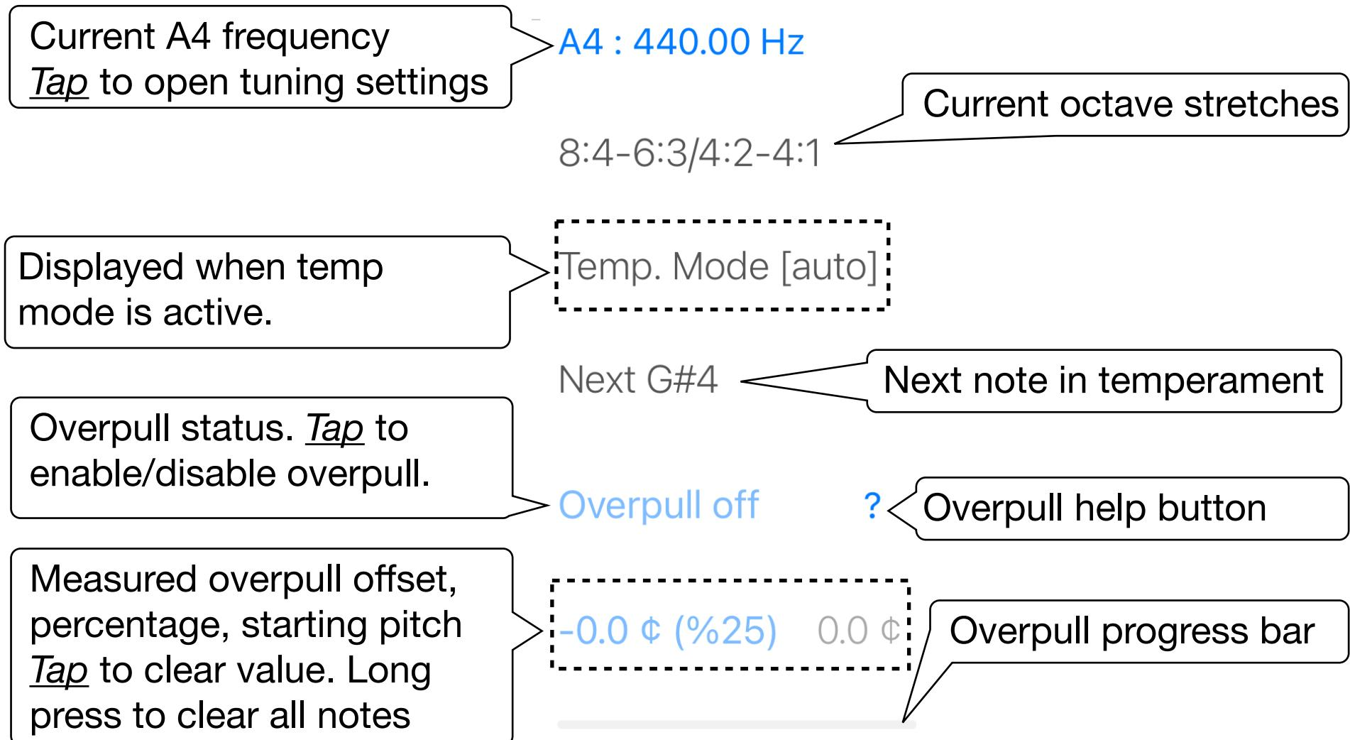
If you set display type to “Minimal”, left and right sections are hidden for a simpler and plain look of the Tuner screen. Minimal display type can be selected if inharmonicity measurements are complete. Over pull can be activated if starting pitch values are transferred from the SP (starting pitch) screen. Double tap to change scale.
