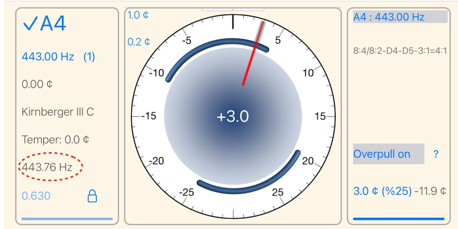
If starting pitch values are not transferred from SP screen (not recommended), in over pull mode **it is important that the note must be briefly measured before being tuned. Pay close attention that over pull measurement is not affected by extraneous noise.**
