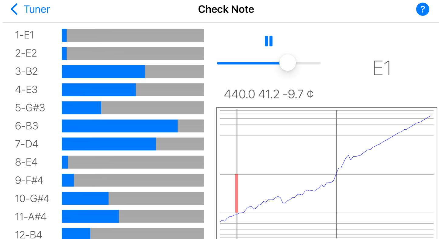
The information might be used for voicing or checking the piano prior to tuning.
