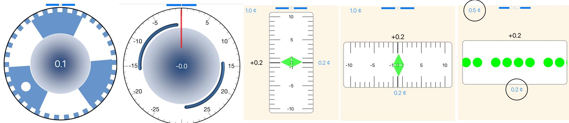
The value in the center of the display indicates the current note's plus or minus cent difference from the target value. If the note is flat the value is minus and the spinner/arcs turn left. With a positive value the note is sharp and the spinner/arcs turn right. When the value is within dial range a red dial indicator is displayed showing the measured value in indicator mode.
