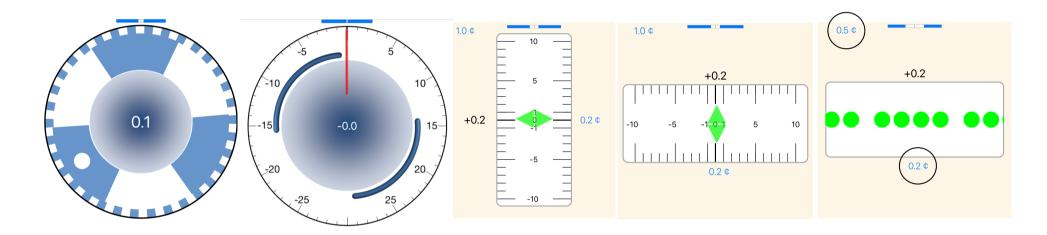
The value in the center of the display indicates the current note's plus or minus cent difference from the target value. If the note is flat the value is minus and the spinner/arcs turn left. With a positive value the note is sharp and the spinner/arcs turn right. When the value is within dial range a red dial indicator is displayed showing the measured value in indicator mode.
