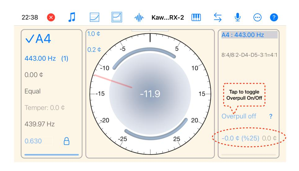
Observe the display when Over pull is ON. Display shows that the note will be pulled by about 14.9 ¢ including the over pull amount.
