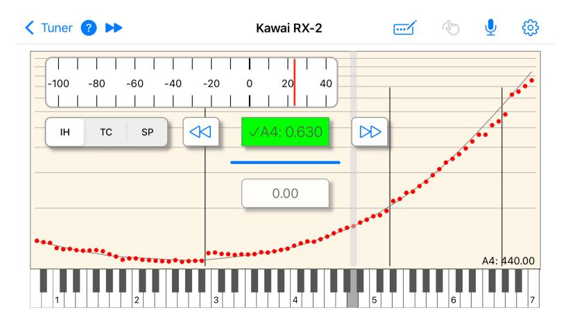
Use horizontal scale to pull up closer to pitch. Swipe up/down to adjust A4 frequency.
