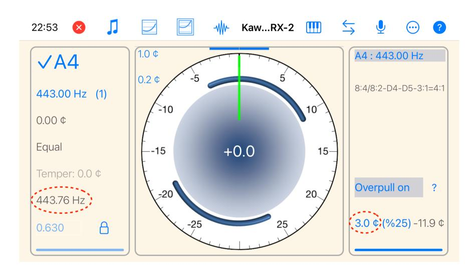
If starting pitch values are not transferred from SP screen (not recommended), in over pull mode it is important that the note must be briefly measured before being tuned. Pay close attention that over pull measurement is not affected by extraneous noise.
