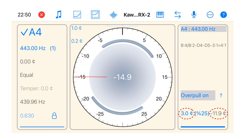
Set Overpull to ON and tune as usual bringing the indicator close to zero. Note that measured frequency reflects the applied overpull amount.
