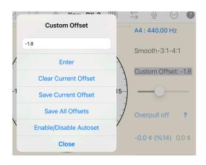
Tap on the offset text to manually enter a value, clear the offset or save the offset(s) as a custom offset in the tuning file and enable/disable auto set. In Auto set you might need to play the note a few times to settle the display to zero cents.
