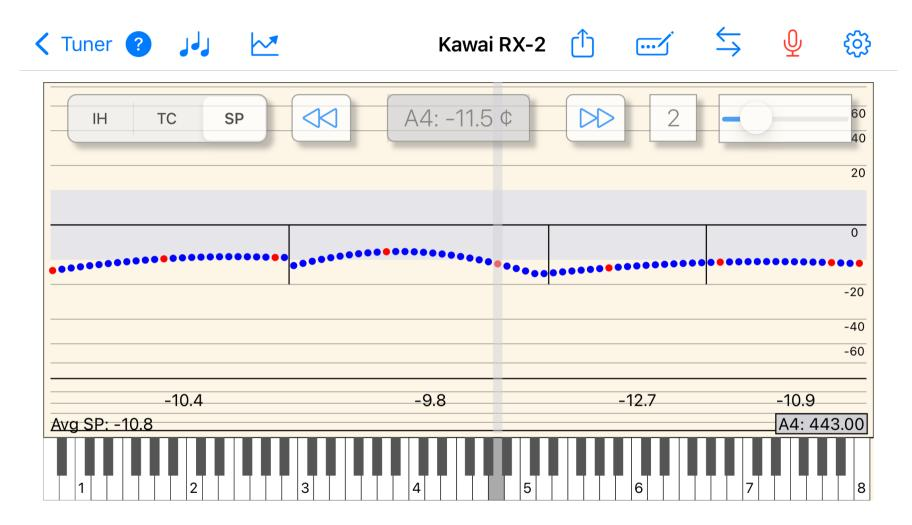
When done, transfer starting pitch values to Tuner screen. A reminder is displayed to set over pull parameters on first use.
