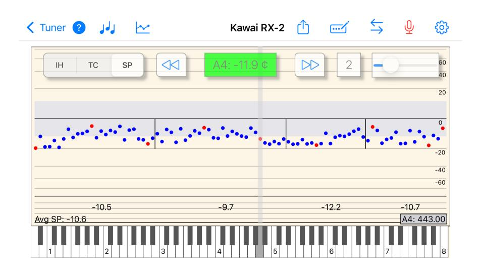
To correct outliers and end up closer to a fine tuning, it is recommended to apply Smooth or Trend on values. A reminder is displayed to set over pull parameters on first use.
