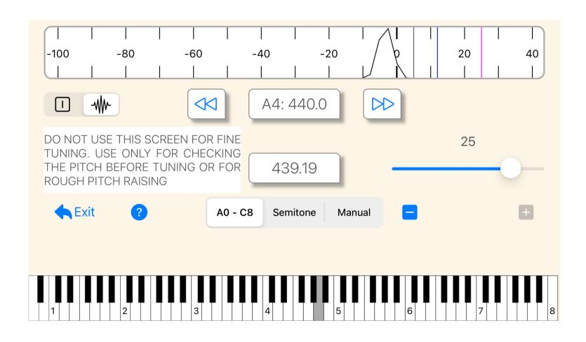
If within 40 cents use the simple start screen to create a new tuning file, and continue with inharmonicity measurement. After completing inharmonicity measurement, switch to Tuning Curve (TC) screen and tap the "Magic Wand" icon to automatically set tuning curve. If over pull is needed, go to Starting Pitch (SP) screen complete measurements and transfer to main screen. Then go to Tuner screen and start tuning.
