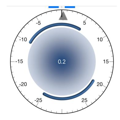
The indicator style can be set to a needle or a triangle through Settings > Display > Indicator Style.
