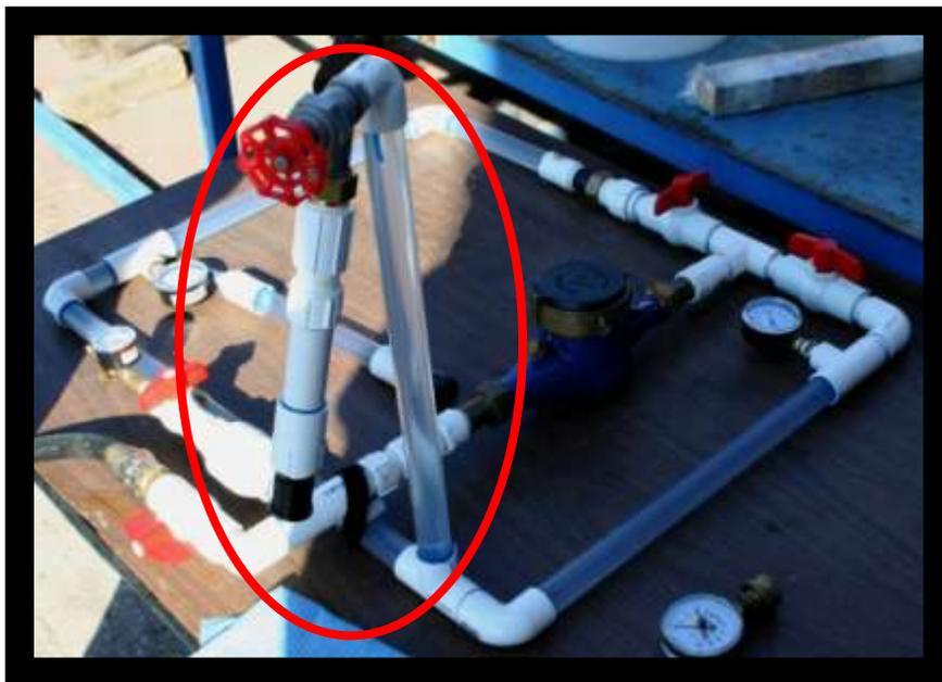
**Figure 6 – Clear Pipe Showing Bubbles in the Water Line**
