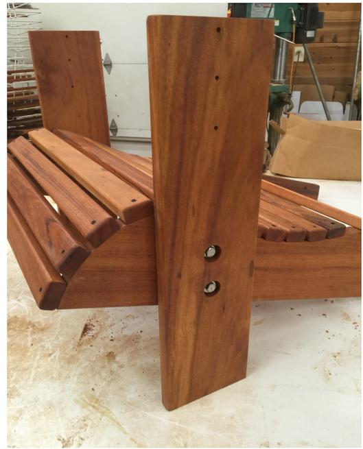
**3-Install Top back support (#6) using 4- 2" screws while centering the 2 rear legs (#5) on screw holes. The front of the rear legs should be flush with front of the top back support**
