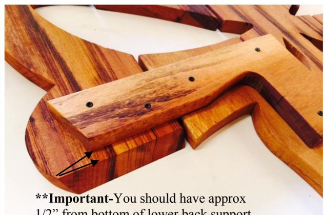
**\*\*Important-**You should have approx 1/2" from bottom of lower back support to edge of bevel
