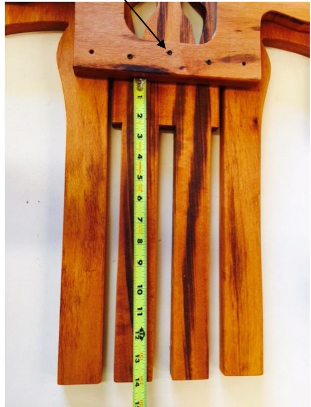
**12-Use a square to be sure the mid brace is perpendicular and centered on the center skull piece #12. As shown here. Pre-drill and install the re-maining center screws.**
