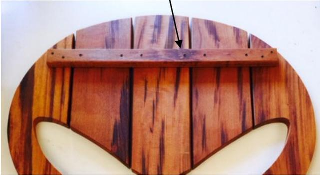
**16**-Install the skull mid brace (#18) on the underneath the top back support. Slide the brace up tight and centered under the back support. Pre-drill and install 6- 1 1/2" thru mid brace and into skull
