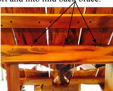
**15**-Lay and center the skull onto the chair. Pre-drill and install 1- 2" screw thru bottom of each arm into the skull, as shown. Making sure the skull is pulled tight to the upper back brace and sitting on each arm equally.
