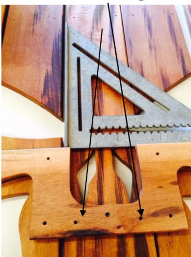
**13-Line up all the remaining pieces so the eyes and top of skull line up. There should be approx 3/8" space in-between all skull pieces. Pre-drill and install remaining screws. The lower back brace should be positioned like this photo**
