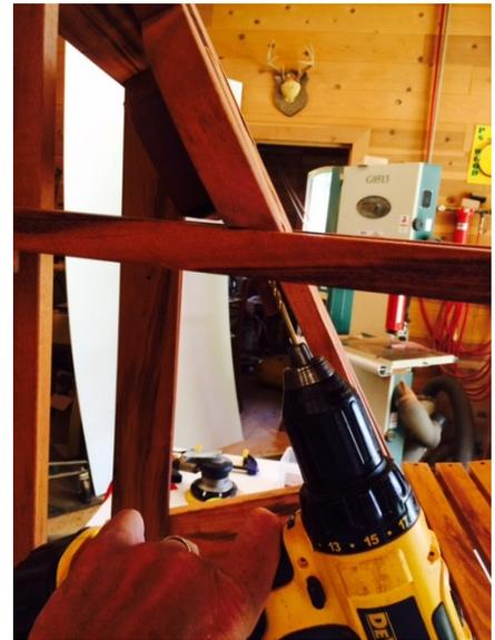
**18**- Pre-drill and install 4- 2" screws thru bottom rear seat slat (#3) and into the fangs or the skull, while pulling the fangs tight to the brace.
