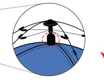
**STEP 4:** After successfully erecting the tent -Push down on the base of the Pop-up Mechanism to to lock the tent in place.
