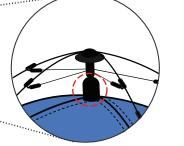
**STEP 6:** To disassemble, first unlock the base of the Pop-up Mechanism by pushing up on it.
