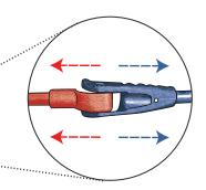
**STEP 7:** To fold the legs back in, pull apart at the joints to unlock the legs. Repeat for all 4 legs of the tent.
