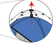
**STEP 3:** After all legs are unfolded, lift up from the Pop-up Mechanism to erect the tent.
