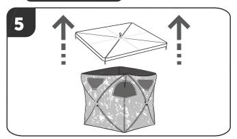
**STEP 5:** To disassemble, first detach and remove the roof of the Hunting Blind. Firmly push in on the web handle to correcity close the roof.
