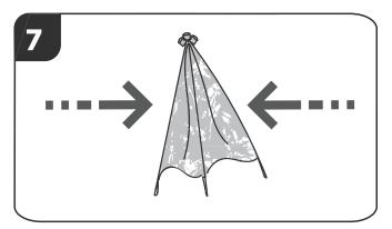
**STEP 4:** After the roof is fully assembled, attach the roof to the top of the Hunting Blind by fastening the buckles located on the corners of the roof and the corners of the Hub.
