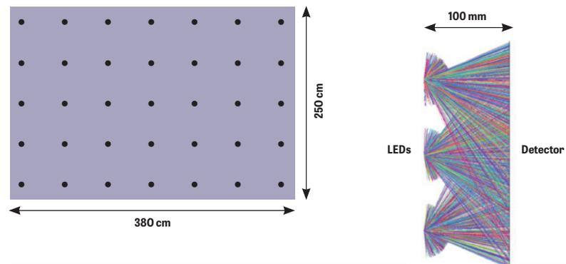
Arrangement of UVC LEDs in the duct.
