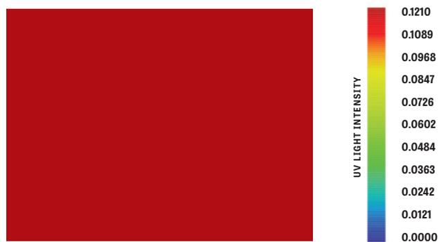
Irradiance model of duct 2 lined with 80% UV reflective materials on all four sides.
