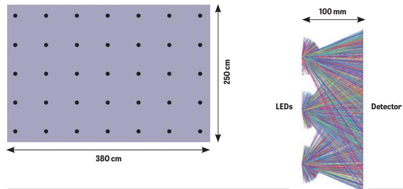
Arrangement of UVC LEDs in the duct.
