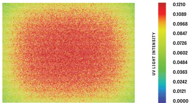
Irradiance model of duct 1 without UV reflective surfaces.
