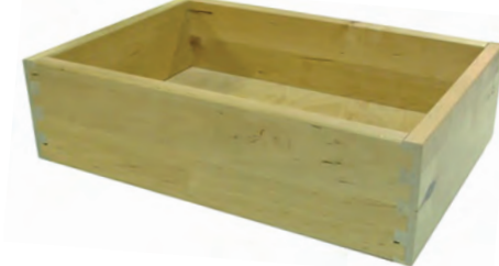
LEVEL 2 Shoulder-Top Finished Dovetail
