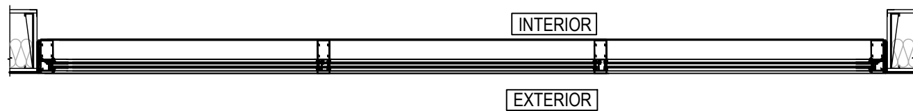
03 WINDOW WALL ELEVATION / QTY: 2 SCALE: 1/2"=1'-0" ARCH. REF. 1 / A301 SYSTEM - 1 (2-1/4" X 6" OFFSET GLAZE FOR 1" GLASS -TC670) S/M: EXTERIOR ELEVATION - NORTH
