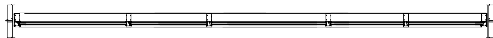
03 WINDOW WALL ELEVATION / QTY: 1 SCALE: 1/2"=1'-0" ARCH. REF. 1/ A301 SYSTEM - 1 ( 2-1/4" X 6" OFFSET GLAZE FOR 1" GLASS -TC670) S/M: EXTERIOR ELEVATION - NORTH
