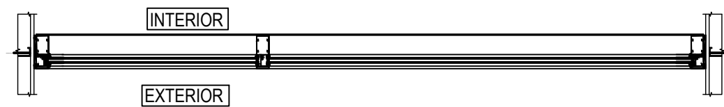
08 WINDOW WALL ELEVATION / QTY: 1 SCALE: 1/2"=1'-0" ARCH. REF. 2 / A302 SYSTEM - 1 (2-1/4" X 6" OFFSET GLAZE FOR 1" GLASS -TC670) S/M: EXTERIOR ELEVATION - WEST
