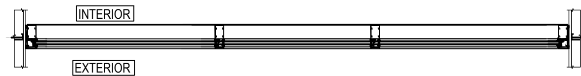
09 WINDOW WALL ELEVATION / QTY: 1 SCALE: 1/2"=1'-0" ARCH. REF. 2 / A302 SYSTEM - 1 (2-1/4" X 6" OFFSET GLAZE FOR 1" GLASS -TC670) S/M: EXTERIOR ELEVATION - WEST
