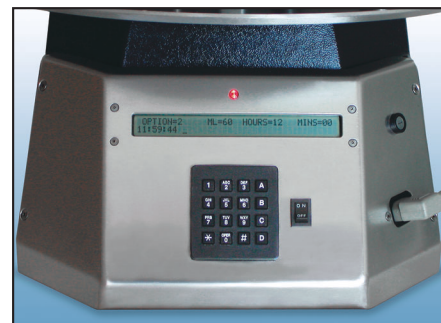
Vacuum Extractor control panel is equipped with an on/off switch, 16 key set-up pad and a red "in operation" indicator.
