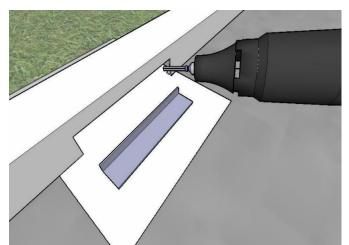
The same setup and cut operation is accomplished on the exterior side of the aluminum flooring member as well.
