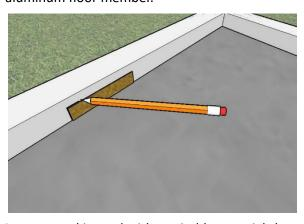
A power tool is used with a suitable one-eighth inch cutting bit to plunge into the 'waste' area and cut just inside the pencil line marked around the template (err on the small side for the opening, file to fit for better results)
