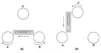
Fig. 6.22 Levelling with three foot screws
