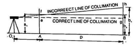
Since the the target is measure with reference to diaphragm (cross hairs + Even if telescope is truly horizontal but reading is slightly different if diaphragm is up or down from centre. So it introduce error in measurement which we called as line of collimation error
