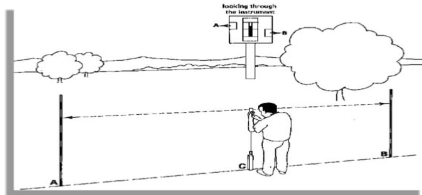
In order to handle the instrument in hand a handle with hook is provided. The hook is to enable a plumb-bob to help transfer the point to the ground.
