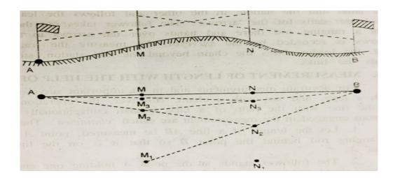
At M1 and N1 two surveyors stay with ranging rods. The person standing at M1 directs the person at N1 to move to a new position N2 as shown in the figure. N2 must be inline with M1B.
