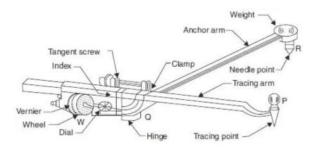
Method 1: the area of the figure is measured in square cm and the field area is determined by multiplying the area of the figure by the square of the scale of the plot. Along with the planimeter, the manufactures supply a scale chart. In this, the positions at which the vernier is to be set on the tracing arm for different scales are given. The vernier is set to a scale of 1:1 and the area of the plot is determined. This is multiplied with the square of the scale to get the field area.
