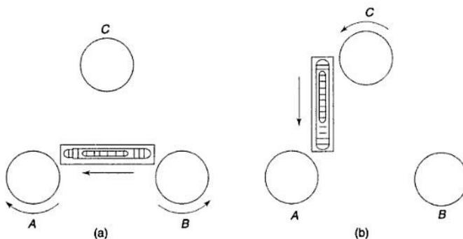
Fig. 6.22 Levelling with three foot screws
