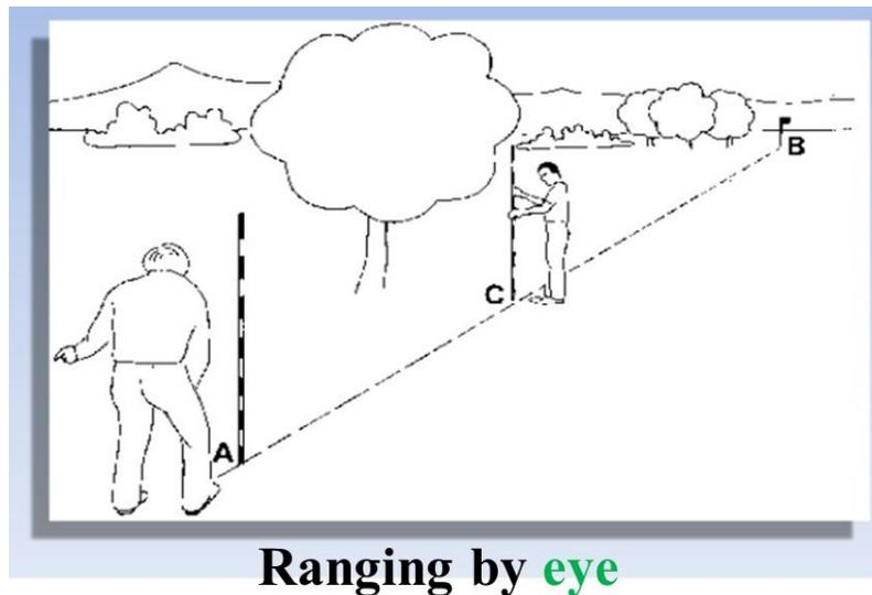
The assistant then takes the ranging rod and establishes at a point in between AB, almost in line with AB. This is fixed at a distance not greater than one chain length from point A.
