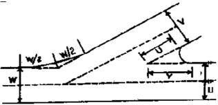
Fig.2. - Rounding off intersection at junctions.
