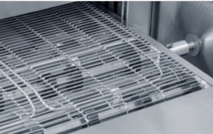
全不锈钢结构,更符合食品卫生要求 All stainless steel structure, comply with food hygiene requirements
