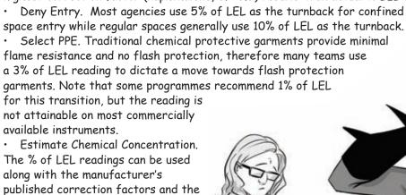
along with the manufacturer's published correction factors and the flammable range of the chemical of interest to calculate concentration. Remember, always calibrate sensors following the manufacturer's guidelines and apply correction factor data specific to the manufacturer and model of the detector you are using.
