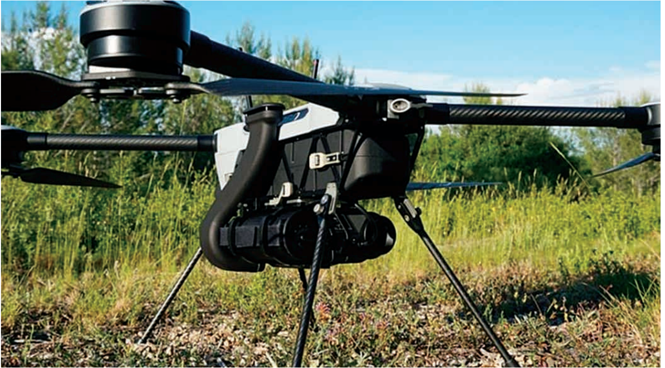
Proengin's new AP4C+ allows it to be mounted on a UAS ©Proengin
