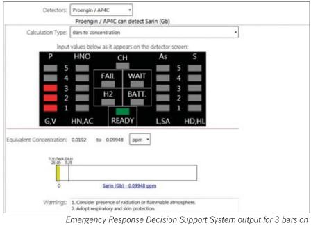
nergency Response Decision Support System output for 3 bars on phosphorous channel of AP4C relative to Sarin ©QFES
