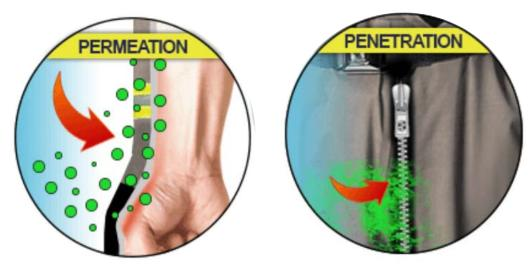
Figure 2: Visualization of permeation and penetration
