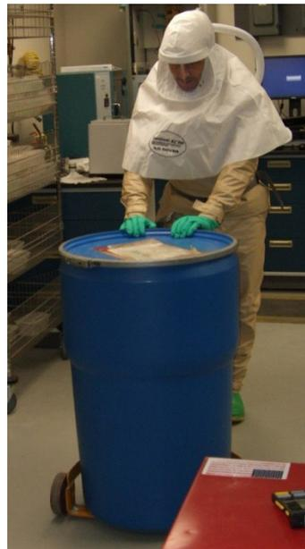
**EXHIBIT 11** Ensemble Being Evaluated for Overall Function by Test Subject Moving 55-Gallon Drum. (Courtesy of Intertek Testing Services.)
