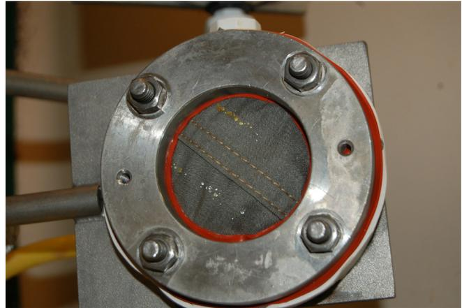
**EXHIBIT 8** Liquid Penetrating Material Samples During Liquid Penetration Resistance Test. (Courtesy of International Personnel Protection, Inc.)
