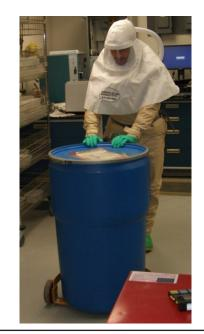
**EXHIBIT 11** Ensemble Being Evaluated for Overall Function by Test Subject Moving 55-Gallon Drum. (Courtesy of Intertek Testing Services.)
