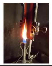
**EXHIBIT 10** Exposure of Ensemble Material in Flame Resistance Test. (Courtesy of International Personnel Protection, Inc.)
