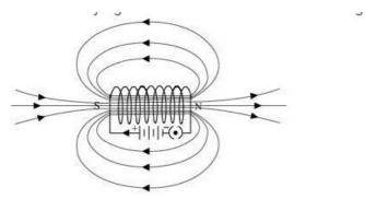
In the above figure, when the north pole of a bar magnet is brought near the end connected to the negative terminal of the battery, the solenoid repels the bar magnet. Since like poles repel each other, the end connected to the negative terminal of the battery behaves as the north pole of the solenoid and the other end behaves as a south pole. Hence, one end of the solenoid behaves as a north pole and the other end behaves as a south pole.
