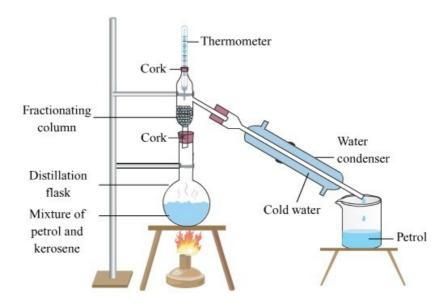
In this method, the mixture of kerosene and petrol is taken in a distillation flask with a thermometer fitted in it. We also need a beaker, a water condenser, and a bunsen burner. The apparatus is arranged as shown in the above figure. Then, the mixture is heated slowly. The thermometer should be watched simultaneously. Petrol will vaporize and condense in the water condenser. The condensed petrol is collected from the condenser outlet, whereas kerosene is left behind in the distillation flask.
