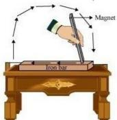
Then, the bar magnet is lifted from the other end and brought to the starting point again with the same pole of the bar magnet. On repeating the process for at least 40 to 50 times, the iron strip will become a bar magnet with two poles.
