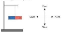
Hence, the unknown poles of a bar magnet can be marked by suspending it freely by a string.
