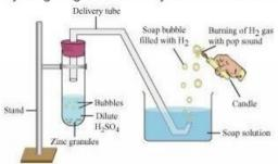
Take few pieces of zinc granules and add 5 ml of dilute H2SO4. Shake it and pass the gas produced into a soap solution. The bubbles of the soap solution are formed. These soap bubbles contain hydrogen gas.
