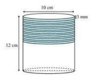
It can be observed that 1 round of wire will cover 3 mm height of cylinder.
