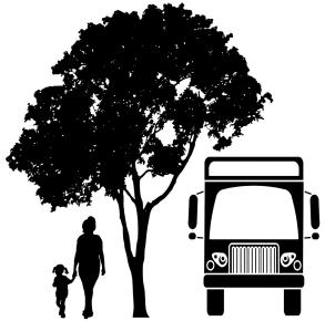
Limbs over the sidewalk shall have a minimum of an 8' clearance
