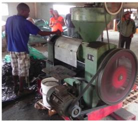
The above photo was taken when the equipment was at another location. With the screw-press machine, seeds are crushed into oil. Afterwards, it is refined and bottled.
