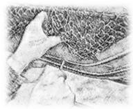
Pull out on the plastic panel and slide the clip removal tool behind it. Locate the tool on each clip securely and use the pry tool to pop the clip off the metal door. You may place a piece of cloth, paper or cardboard between the tool and the metal door to protect the paint on the door.
