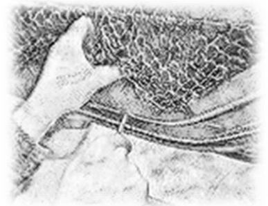
Pull out on the plastic panel and slide the clip removal tool behind it. Locate the tool on each clip securely and use the pry tool to pop the clip off the metal door. You may place a piece of cloth, paper or cardboard between the tool and the metal door to protect the paint on the door.
