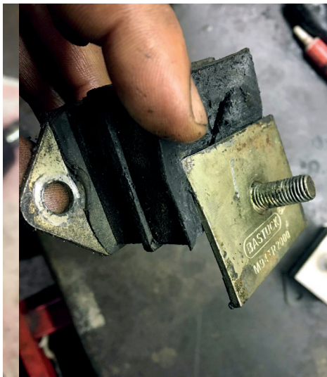
Perished engine mounts are now removed
