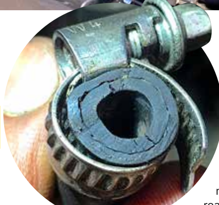
Hoses looked OK-ish on the outside, but inside... unsafe.
