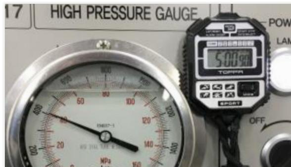
The original specimens were subjected to all three Pneumatic Proof Tests and all three Hydrostatic Proof Tests (including 10 repeat assemblies), concluding with the Hydrostatic Burst Test (destructive test). New specimens were introduced for each of the remaining test.
