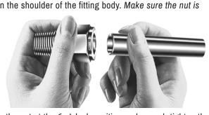
Step 2.) Scribe the nut at the 6 o'clock position and wrench-tighten the nut 1+1/4 turns to the 9 o'clock position, holding the body with a backup wrench. Tighten the nut 3/4 turn to the 3 o'clock position for 1/16", 1/8", and 3/16" - 2, 3, and 4 mm Tube Fittings.
