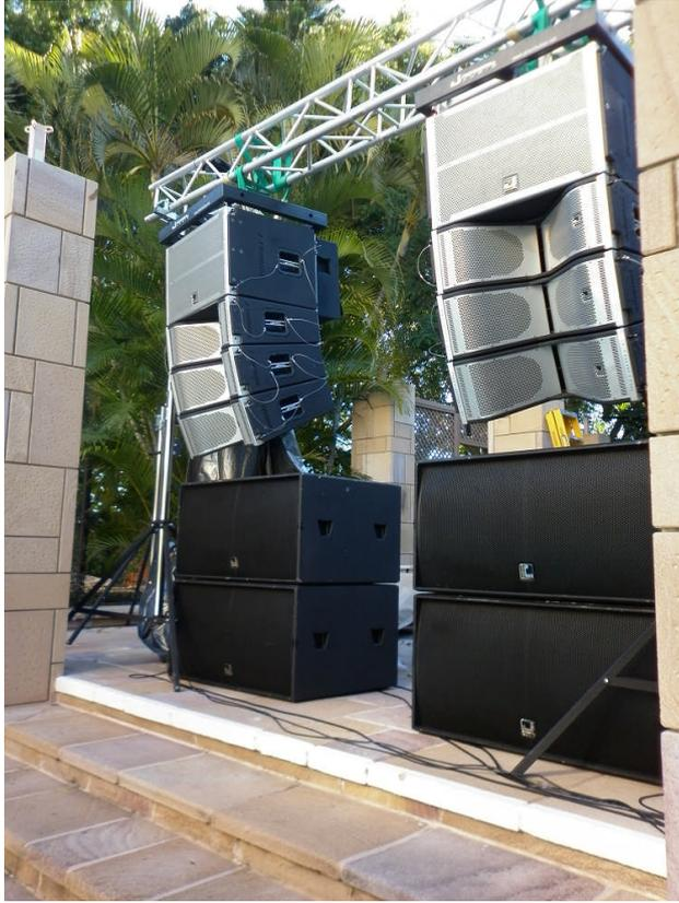
**Figure 3 – Line Array sound system (front view)**
