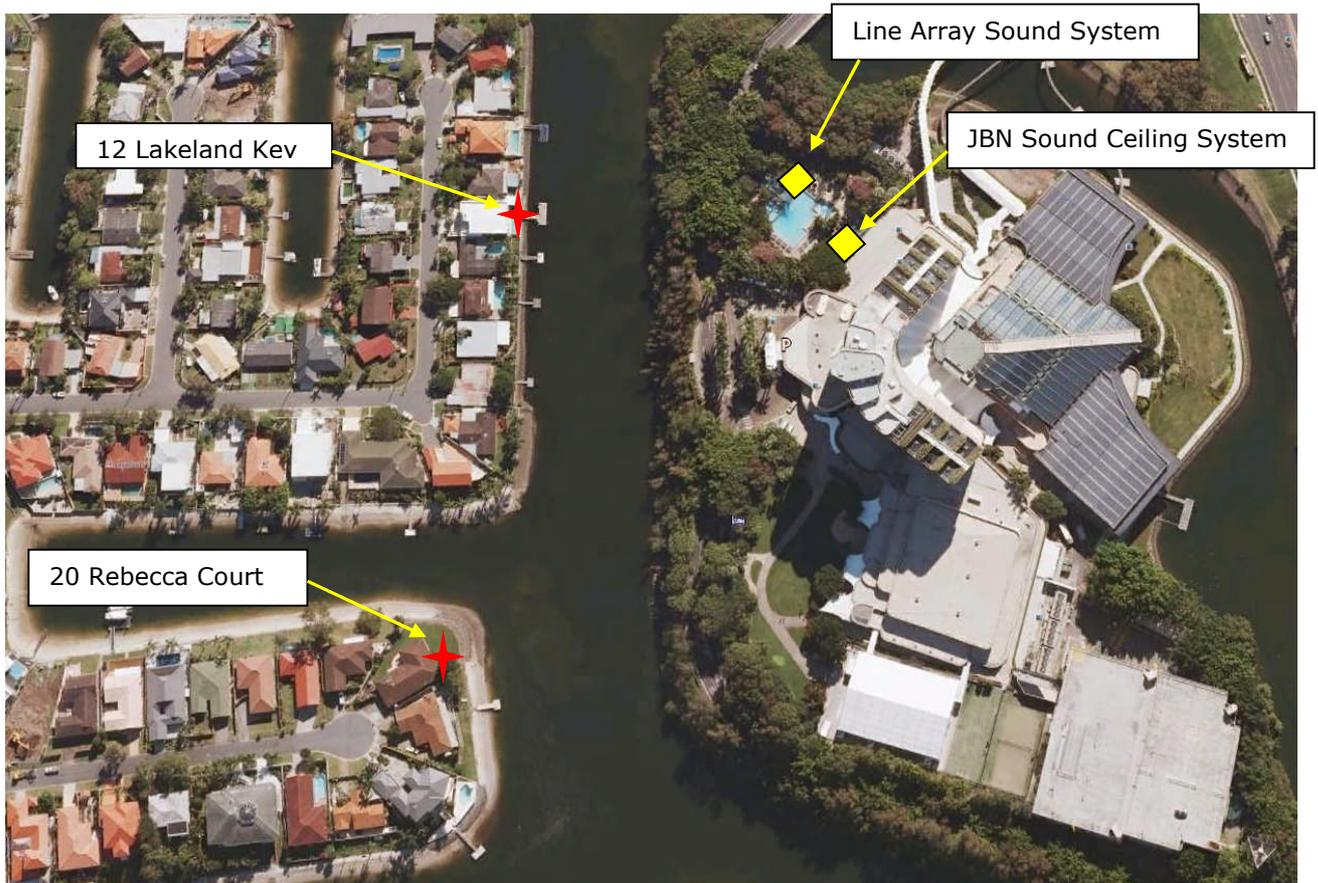
**Figure 9 – Speaker System Locations & Residential Measurement Locations**
