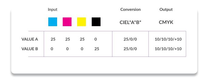
Here, you can see how the results from a CIEL\*A\*B\* conversion differ to the results we see if Values A and B are converted directly from CMYK-to-CMYK. Less ink gets laid down as part of value 1 in comparison to value 2, which means a less vivid color is the output. Colors get contaminated In the CIEL\*A\*B\* space, which sees both values as being equivalent and therefore converts these to identical outputs. Quite simply, the output isn't what was intended.
