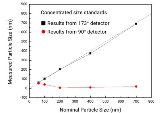
When the sample is detected at 173° at the middle of the cell, the scattered volume is 8-10 times larger than at 90°, leading to much higher sensitivity, and avoiding reflections from the sample cell wall.
