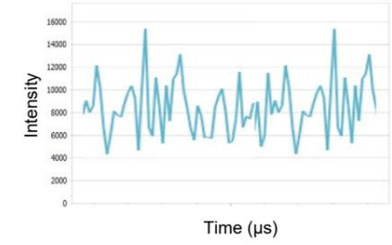
Intensity Fluctuations of Large Particles
