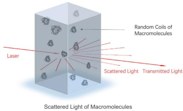
Static light scattering (SLS) is a technology that measures the scattering intensities, weight-average molecular weight ( $M_w$ ) and second virial coefficient ( $A_2$ ) of the sample through Rayleigh equation:
