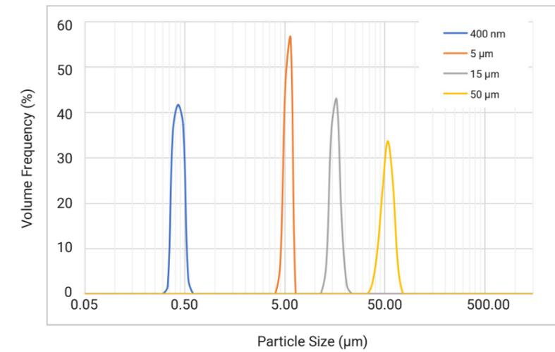
Duke standard samples were measured separately by the Bettersizer ST, showing the distribution peak in the correct position and narrow distribution with high accuracy.
