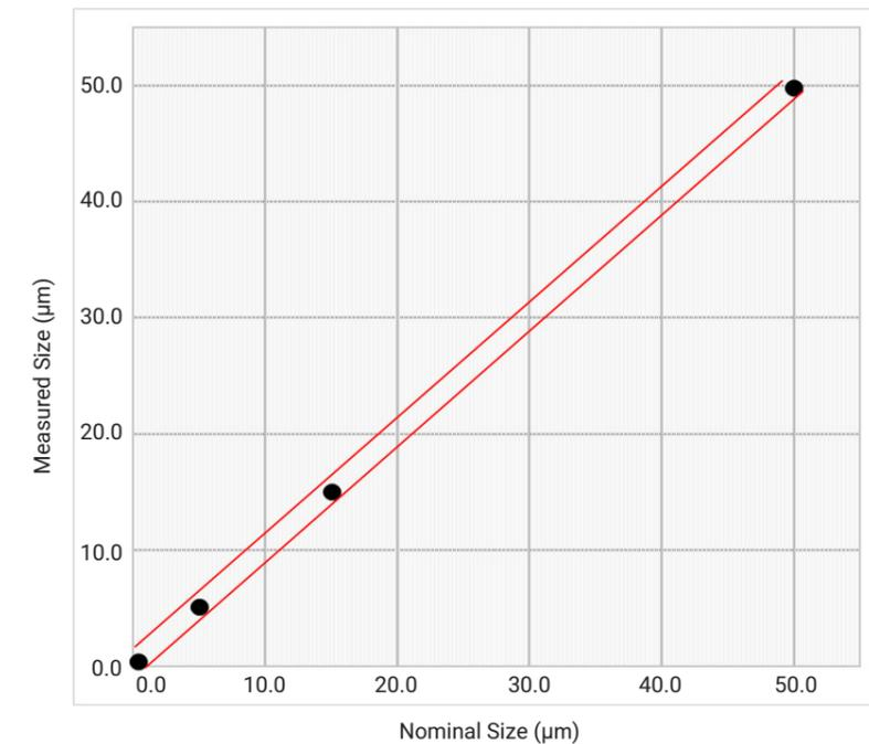
The red line is the nominal size range of standards  $\pm 1.0\%$ , and the black dots are the measured sizes. As shown in the figure, the measurement accuracy of Bettersizer ST for standards is within 1%.
